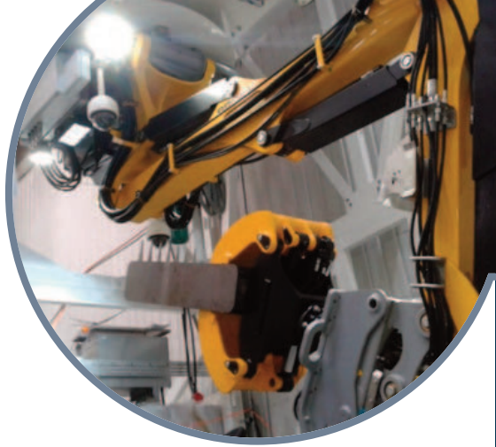
Robotic waste retrieval system.
